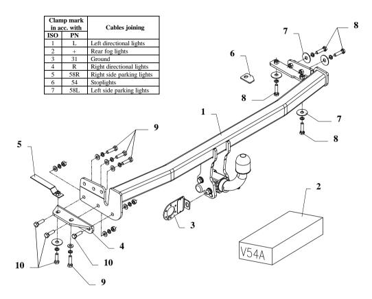
This towbar is designed to assembly in following cars: **NISSAN PRIMERA P 11 4/5 doors,** produced since 10.1996 till 08.1999, catalogue no. **V54A** and is prepared to tow trailers max total weight **1700 kg** and max vertical load **75 kg**.
