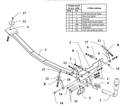
This towing hitch is designed to assembly in following cars: **FIAT TIPO, 3/5 doors,** produced since 1988 till 1995, catalogue no. **R03** and is prepared to tow trailers max total weight up to **1200 kg** and max vertical mass **75 kg**.
